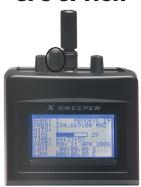
The X Sweeper has an optional GPS receiver and antenna. The GPS receiver module and antenna are factory installed inside the X Sweeper The GPS option displays the Latitude and Longitude coordinates of the X Sweeper location at the time it detected a signal .
