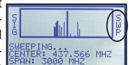
There are 10 different sweep spans (3GHz, 1GHz, 300MHz, 100MHz, 30MHz, 10MHz, 3MHz, 1MHz, 300kHz and 100kHz). If the center frequency was entered as 400 MHz and sweep span was selected as 100MHz, the X Sweeper would sweep from 350MHz to 450MHz and display any signals outside this range would not be displayed.
