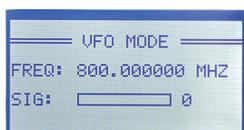
Tune to a specific frequency by entering that frequency directly into the keypad while in VFO mode. A frequency may be stored and then manually locked out in MEMORY mode.
