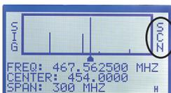
The X Sweeper has the ability to scan frequencies already saved to memory helping to determine if frequencies captured previously are still active.
