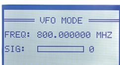
Tune to a specific frequency by entering that frequency directly into the keypad while in VFO mode. A frequency may be stored and then manually locked out in MEMORY mode.
